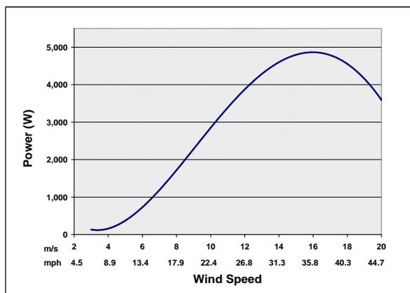
\*Power curve data measured with appropriate load
